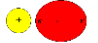
Upon approach of an ion, the electrons in the atom respond and the atom develops a dipole.
