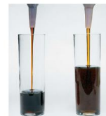
SAE 40 higher number higher viscosity slower pouring SAE 10 lower number lower viscosity faster pouring
